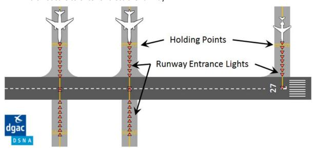
2. Take-off Hold Lights (THL): Sets of red lights illuminating along the axis of a runway in front of a departing aircraft when it is unsafe to take-off from that runway due to an obstacle (vehicle or aircraft) already occupying the runway ahead.
